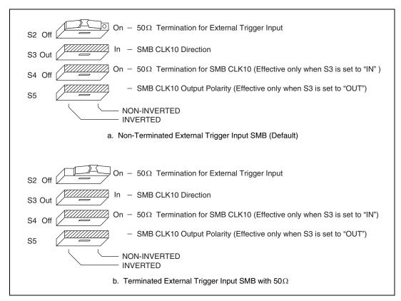
Figure 3-8. SMB Trigger Input Termination
